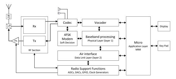
Figure 1: Typical Digital Radio Function Block Diagram
