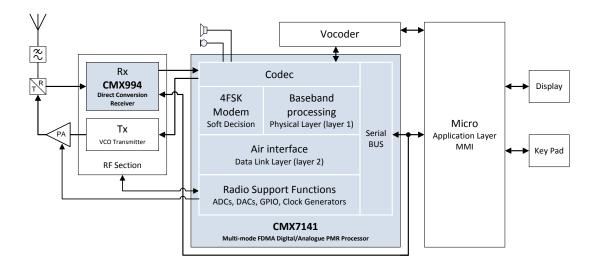
Figure 2: CMX7141 and CMX994 - The Ultimate FDMA Digital/Analogue Radio Chipset
