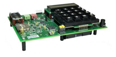
Figure 3: DE9944 SDR FDMA Radio demonstrator
